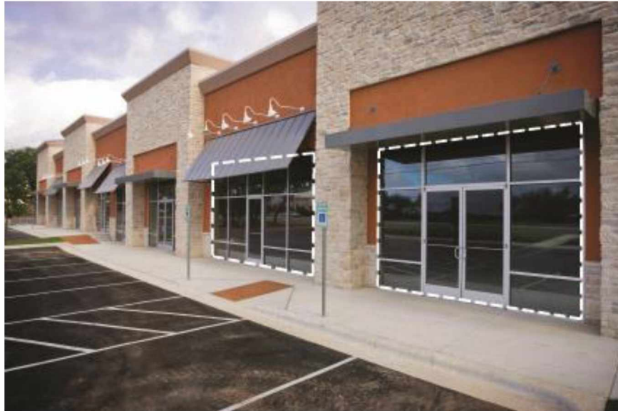
Figure 16: Dashed line on the two storefronts in the above image indicate window area. The dashed lines highlight two separate window areas due to the separation by an architectural feature not related to the windows.
