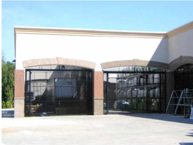
Figure 6: The above image illustrates a wall and fence that is an extension of the principal building that is designed to screen outdoor storage areas.
