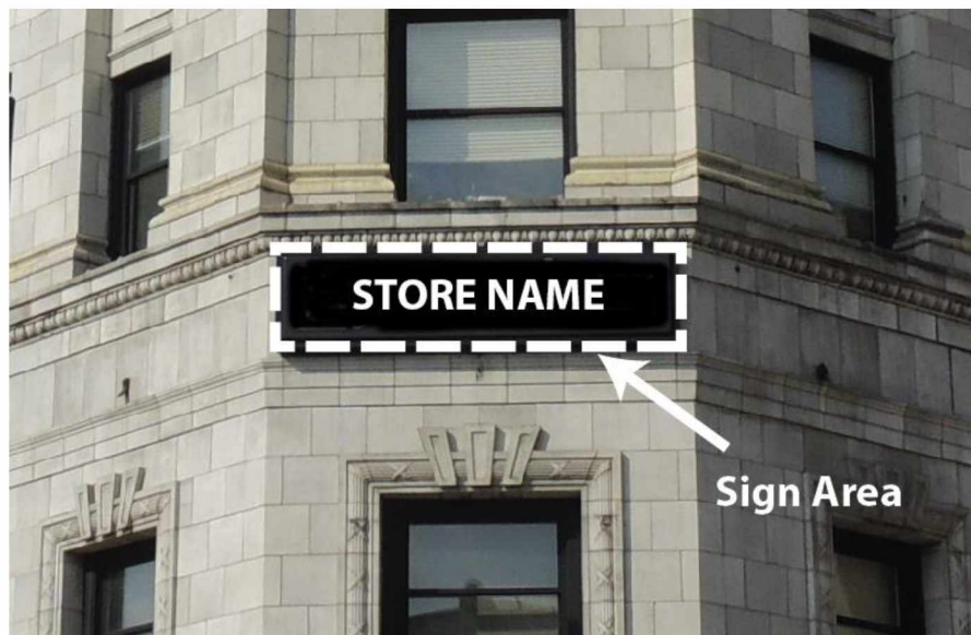
Figure 10: Illustration of computing the sign area for wall signs with a background panel or cabinet
