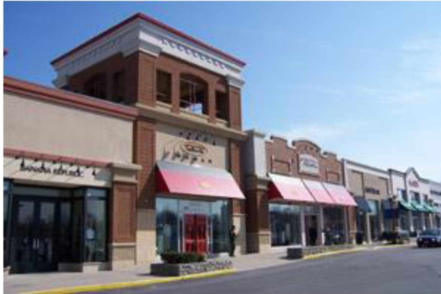
Figure 18: The above image illustrates material changes, pilasters, and other architectural features break up the appearance of a single facade.
